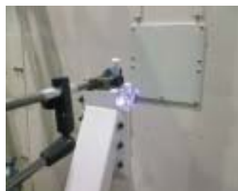
Fig. 2. CPL-UV irradiation of amino acid solution.
