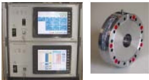
Fig. 1. Charge integration and automatic injection module (left), Integrating Current Transformer (right).
